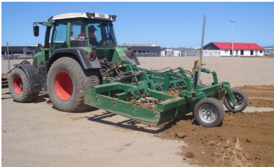
Land levellers and the LB4 dual grade laser
